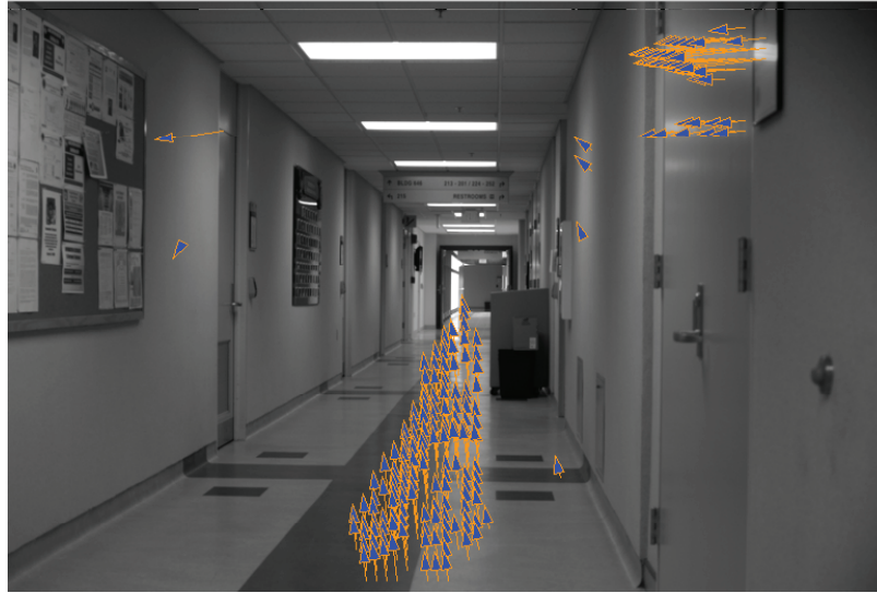
Figure 4.7: Typical hallway results for the standard deviation of a sliding window test. The arrows show the places that were determined to be locally flat and are pointed in the direction of the surface normal. Arrows in the image may be pointing in a direction opposite to the surface normal due to the ambiguity of the angle of polarization.
